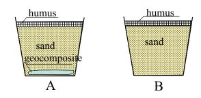
Fig. 3. Arrangement of humus, sand layers and SAP geocomposite position for preliminary application tests: A – container with a strip of geocomposite containing SAP; B – control container without superabsorbent; layers thickness: humus – 20 mm, sand –300 mm, geocomposite – ca. 50 mm.
