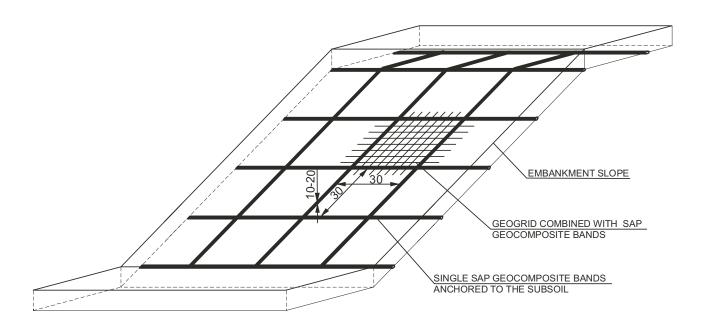
Fig. 7. Possible arrangements of geocomposite with SAP applied on slopes.
