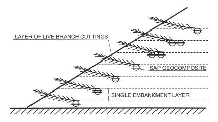
Fig. 8. Application of geocomposite with SAP on a slope with live branch cuttings.
