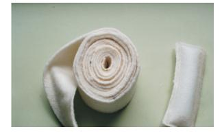
Fig. 2. Gecomposite made of non-vowen geotextile with superabsorbent (SAP). On the right – small strip of the geocomposite swelled after water has been absorbed.
