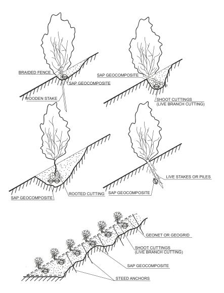
Fig. 9. Application of SAP geocomposite in terrace protection.
