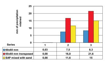
Fig. 1. Additional retention of water from precipitation in sand with SAP for different SAP arrangement in a column test. Theoretical sorption possibilities of SAP amount used in tests – 30 mm of rainfall.
